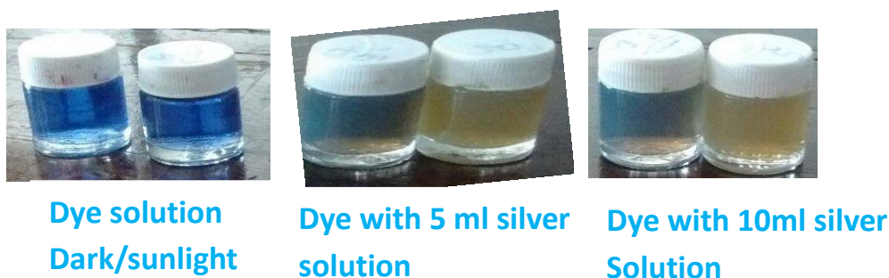
Fig 3: Comparison of dye and dye with silver solution kept in dark and after irradiating with sunlight for 2 hours
