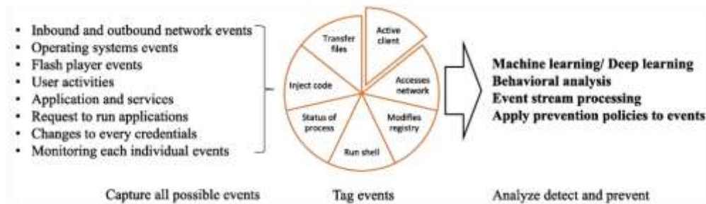
Fig: 4, A framework to detect & prevent fileless malware attack
