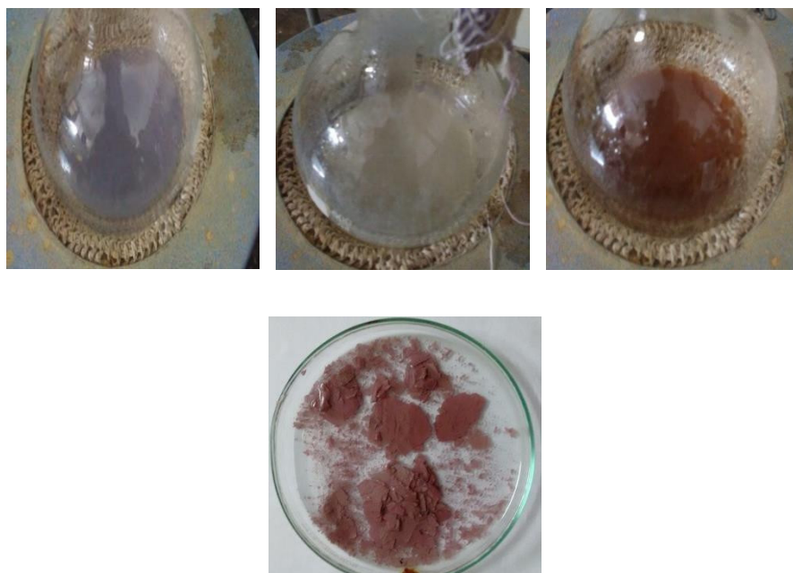
Figure 1: Colour transformation of the sample prepared via Chemical synthesis method
